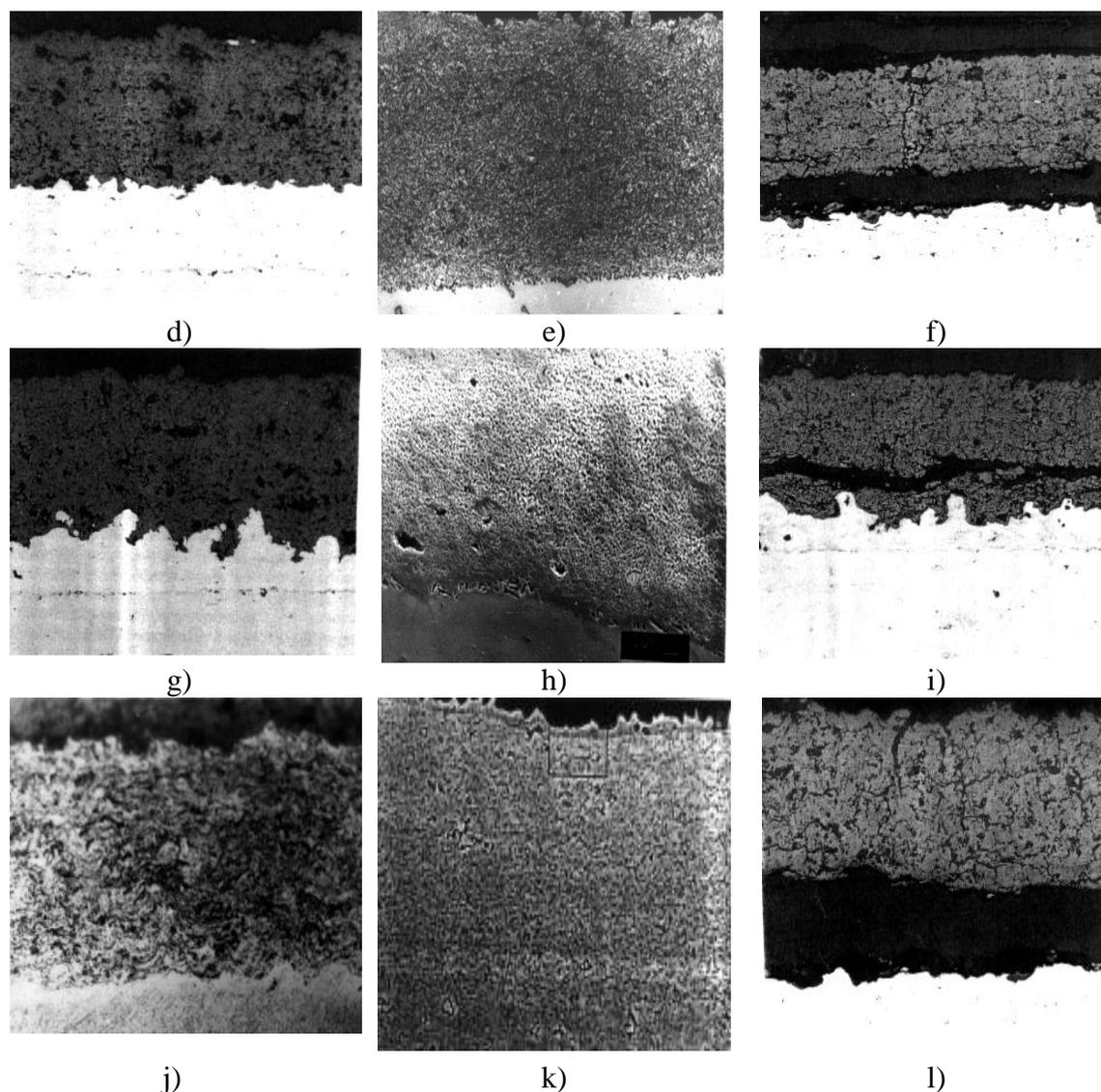
**Figure 1.** Microstructure of heat-shield coatings of the NiCrAlY-ZrO<sub>2</sub>-7%Y<sub>2</sub>O<sub>3</sub>. 400. a), b), c) - APS; d), e), f) - SAPS; g), h), i) - VPS; j), k), l) - HVOF; a), d), g), j) - coating after deposition; b), e), h), k) - coatings after thermal treatment (1100 °C, 2 hours - vacuum); c), f), i), l) - coatings after thermal cycling (heating up to 1170 K, holding for 15 minutes, cooling down to room temperature with compressed air).
