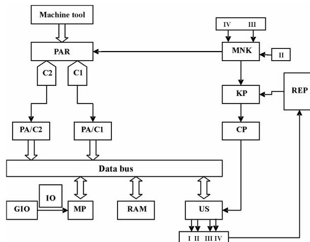
Fig. 4. Diagram of controlling system of elastic-deformable state basing on microprocessor
