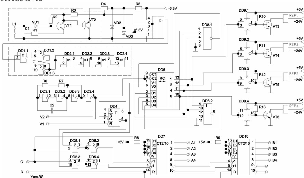
Fig. 5. Schematic diagram of the system of controlling the winding gear basing on the walking pneumatic drive
