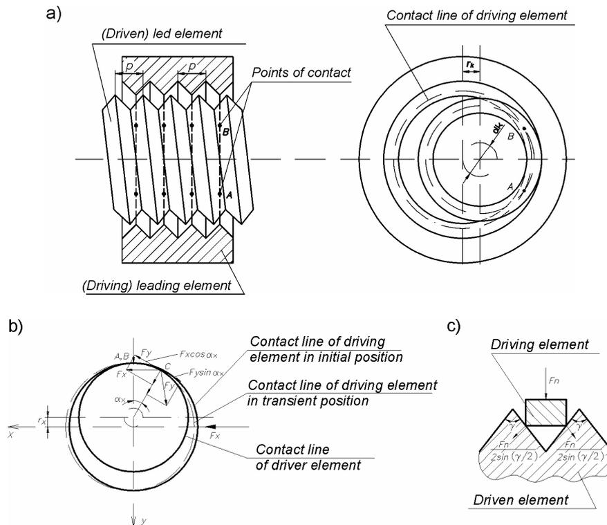
Fig. 2. Computational diagram of vibratory walking pneumatic drive: geometry of driving and driven elements' co-operation – a; scheme of driving and driven elements' contact – b; scheme of applying the component of force on the side of the drive
