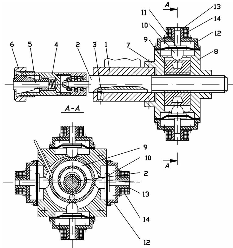
Fig. 1. The tailstock with vibratory walking pneumatic drive
