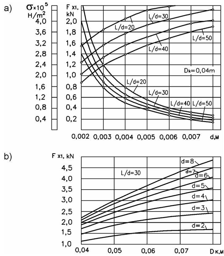
Fig. 3. Relationship between tensile force and normal stresses by different part's diameters  $D_k=0,04m$  – a; change of tensile force by change of pneumatic chamber's diameter – b
