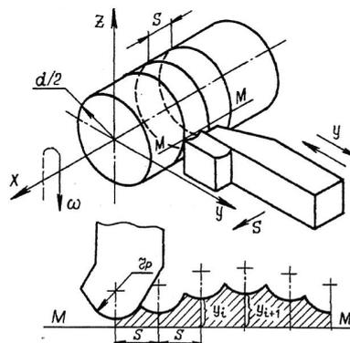
Fig. 1. Diagram showing irregularity at rolling formation, where M\_M is a route of the profilogram;  $y_i$  and  $y_{i+1}$  is a mutual parts and blades movement sizes.
