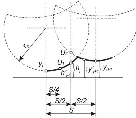
Fig. 2. Scheme of putting the blade profile to modeled profilogram ( $s=f$ )
