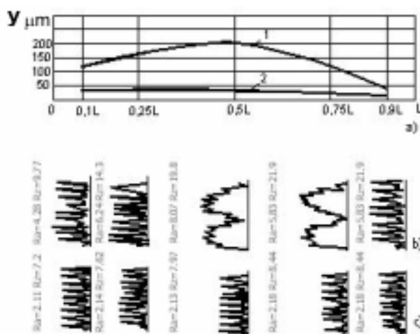
Fig. 3. Relation of elastic strains change in the shaft processed across the length: a) 1-d=10mm curve,  $L=200mm$ ,  $f=0,1mm/ob.$ ,  $v_c=3m/s$ ,  $a_p=1mm$ ,  $\kappa_r=45^0$ ,  $r_p=0,15mm$ ; curve 2 -  $d=20mm$ ,  $L=200mm$ ,  $f=0,1mm/ob.$ ,  $v_c=3m/s$ ,  $a_p=2mm$ ,  $\kappa_r=45^0$ ,  $r_p=0,15mm$ ; b) roughness characteristics change at turning  $d=10mm$  shaft; c) roughness characteristics change at turning  $d=20mm$  shaft
