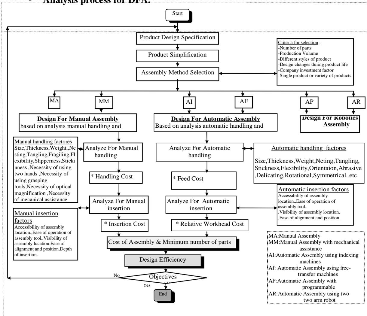
Fig. 2 Proposed analysis process for DFA
