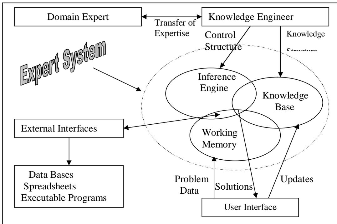
Fig. 1. Integration of Expert Systems Components
