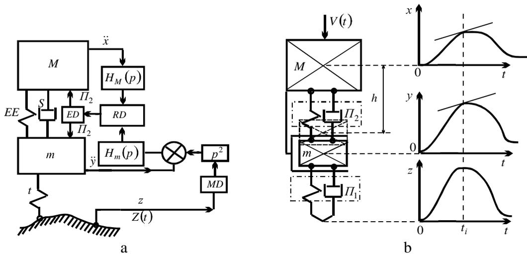
Fig. 1. The scheme of an active suspension of the vehicle (a) and classical two mass system with the limited general movement of a suspension (b):
